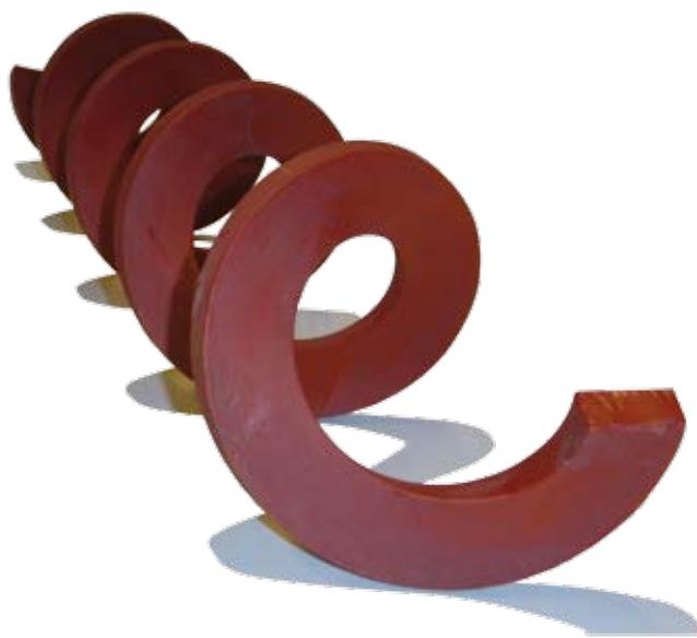
Shaftless spirals are available in lengths between 3.000 and 4.000 mm. (material ST 52.3 and stainless steel 304). Spirals may be used for horizontal, inclined, or vertical conveyor purposes.
